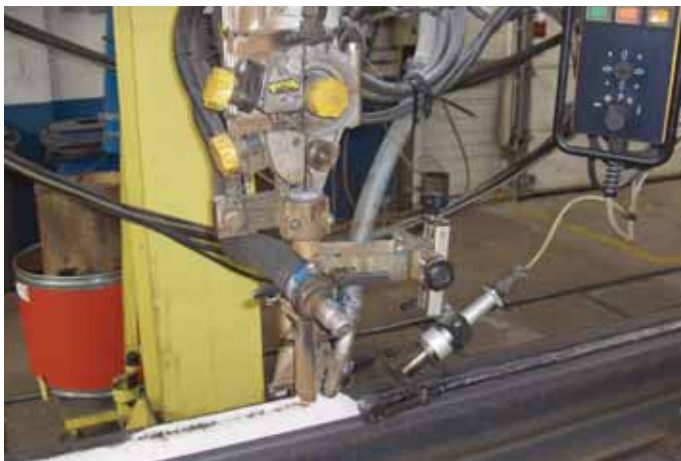
Automatic build-up welding - STIB
