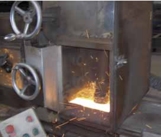
Grinding after build-up welding - STIB
