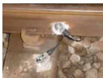
Vibration sensors installed on rail and sleeper (left picture) and vibration sensors installed on concrete structure (right picture)
